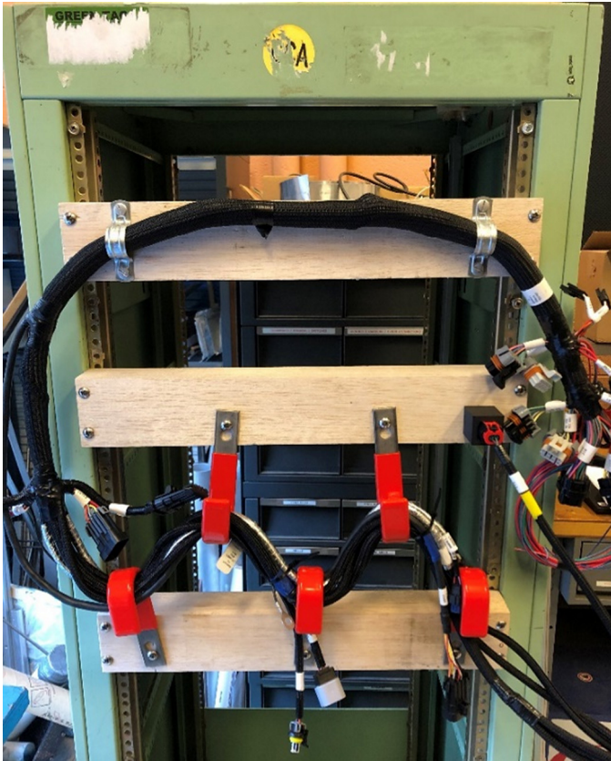
Figure 1. The mock electrical cabinet after the Manipulation Experiment. The bottom half of the wire harness shows the zip ties used to secure its branched ends (steps 1 and 2). The top half features u-brackets for screwing the wire harness onto the cabinet (step 3). Red hooks were used to route the wire harness (step 4), and a three-dimensional (3-D)-printed socket above the rightmost hook allowed subjects to plug in the wire harness connector (step 5).
